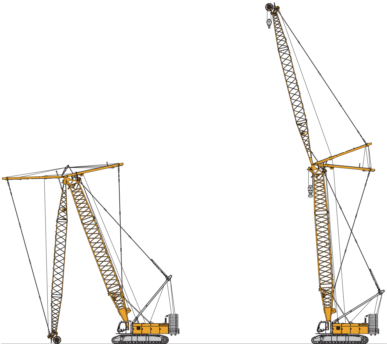
Erecting of main boom and luffing jib
